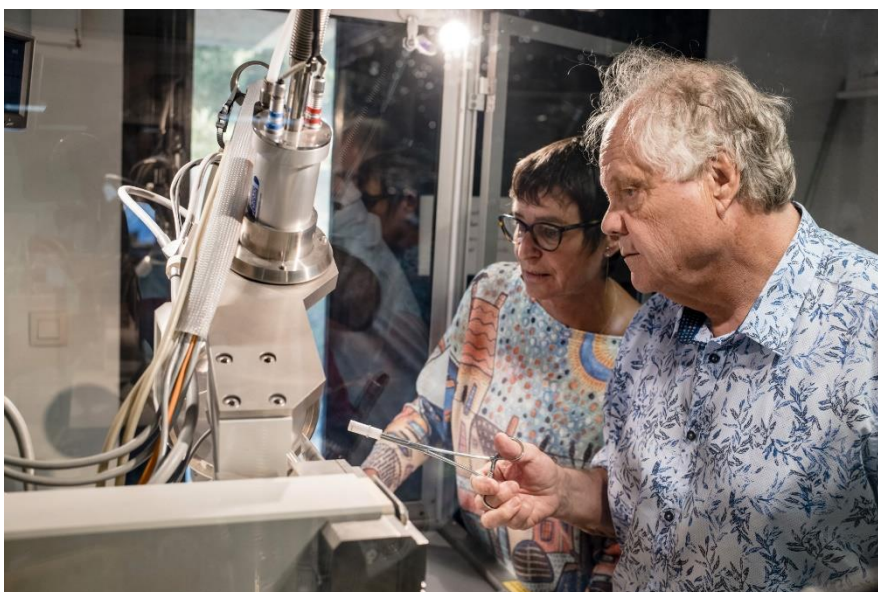
Claverie and Abergel work on an X-ray diffraction device used to determine the 3D structure of viral proteins. Photographer: Jeremy Suyker/Bloomberg
